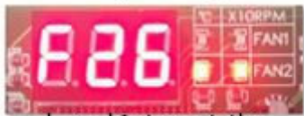
channel 2 stop-rotating temperature
