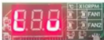
too low voltage
