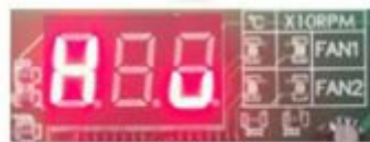
too high voltage
